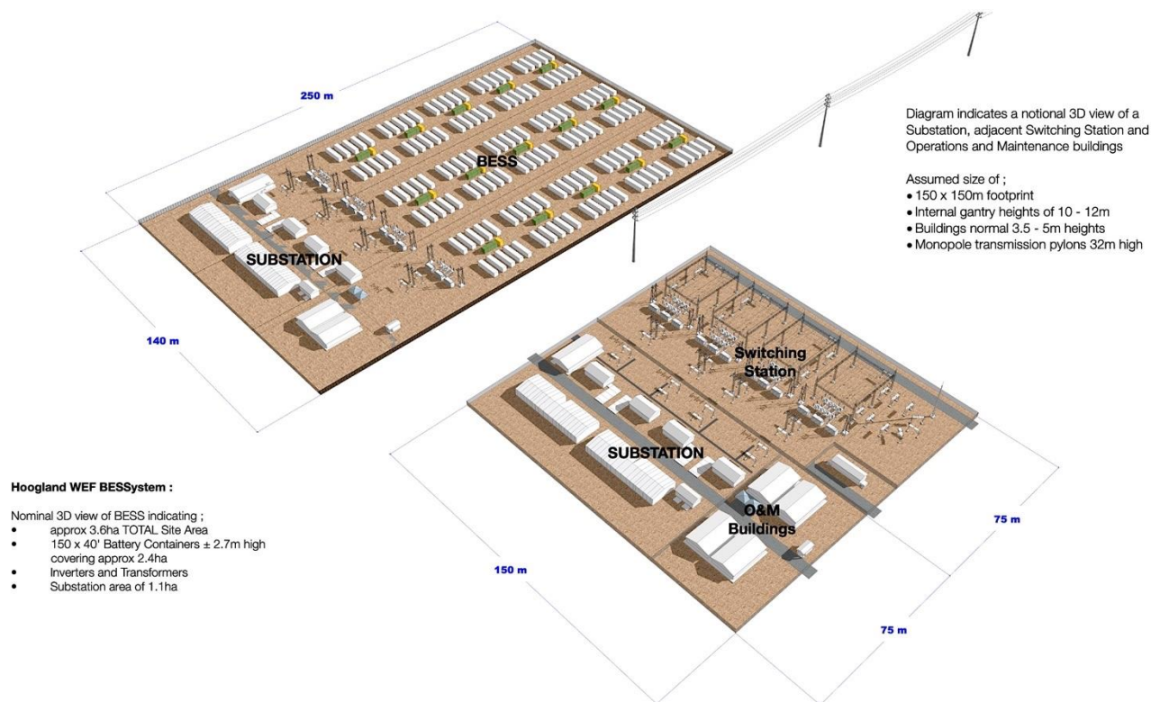
Figure 6: Indicative layout of BESS (Lithium ion, with substation), substation and switching station
